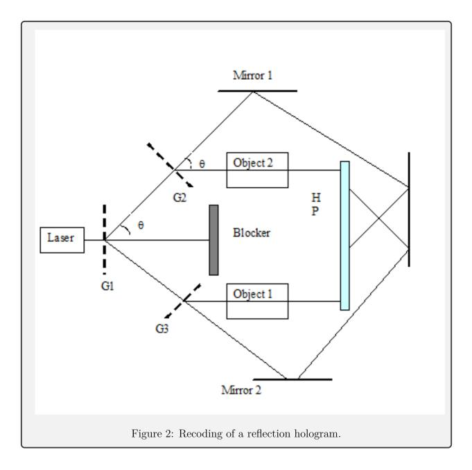
Singh /ISTJN 2015, 6:69-74. Beam method for recording transmission or reflection holograms
